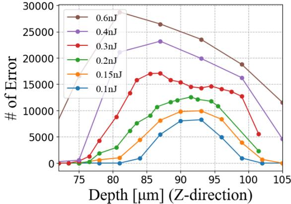
Fig. 2. Number of error under test performed in different depth and energy
