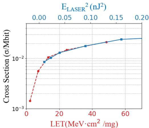
Fig. 3. Cross Section ( $\sigma/\text{Mbit}$ ) of TPA laser (Blue-Slid) and heavy ion (Red-Dashed)
