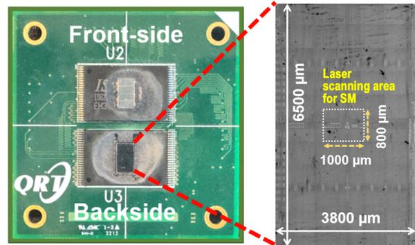
Fig. 1. DUT for laser and heavy-ion evaluation, Entire SRAM IR image for PL and heavy-ion evaluation with laser scanning area for SM
