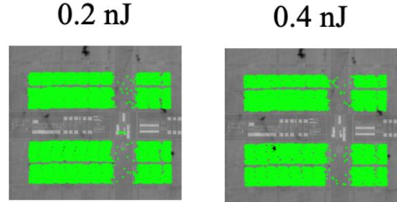
Fig. 4. Sensitive map of 65nm SRAM drawn for different Energy
