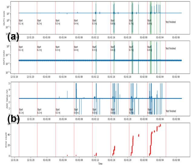
Fig.4. SEE visualization by error mapping on front side chip
