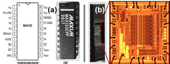
Fig.1. Pin configuration (a) & front de-capsulated MAX153ADC (b)
