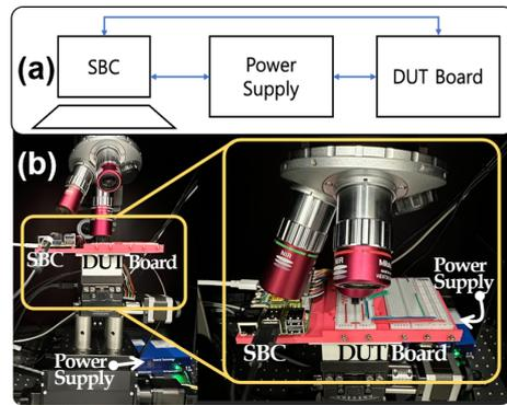
Fig. 2. LASER EVALUATION SETTING: (a) Block diagram of the testing setup, (b) Evaluation system based on (a).
