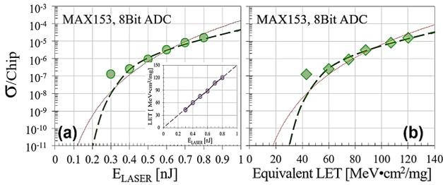
Fig. 3. (a) Cross-section ( $\sigma$ ) of MAX153 irradiated front-side chip with many laser-energy conditions and (b) Converted heavy ion cross-section ( $\sigma$ )
