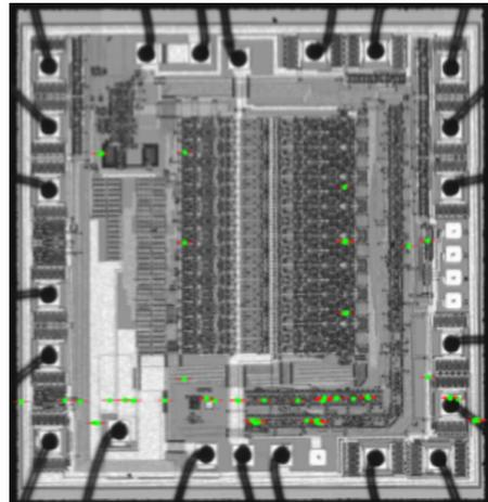
Fig. 5. Error location of MAX153 ADC
